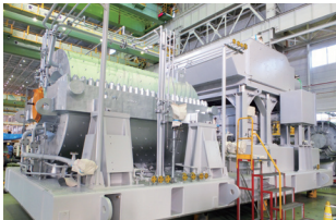
Main refrigerant compressor for LNG plant
