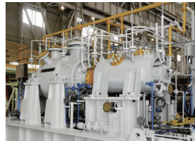
Gas injection compressor for FPSO
