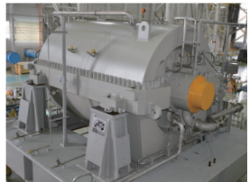
Product gas compressor for PDH plant
